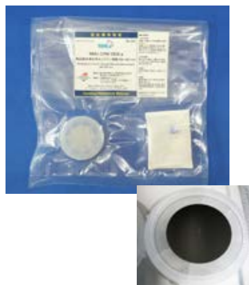
NMIJ CRM 5808-a 熱拡散率測定用 モリブデン薄膜 (400 nm) Molybdenum Film for Thermal Diffusivity Measurement (400 nm) (p. 43)
