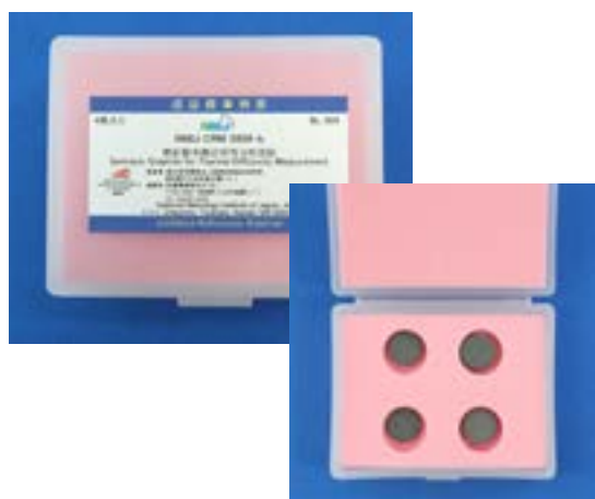
NMIJ CRM 5804-b 熱拡散率測定用 等方性黒鉛 Isotropic Graphite for Thermal Diffusivity Measurement (p. 43)
